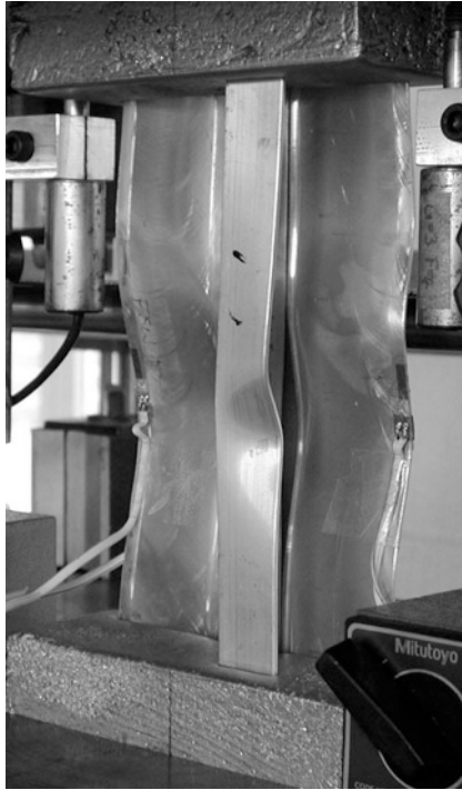
Fig. 8 Validation specimen crippling. The figure illustrates the ultimate failure mode of validation specimen FSW-2 prior to the removal of applied loading.
